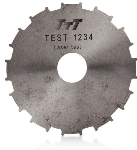
You can generate dark codes without engraving the metal by using an annealing effect
