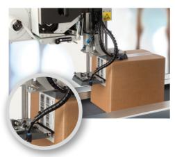
Where larger label information needs to be printed and applied to products or secondary packaging, the M-Series print and apply labelling range offer flexible solutions for full GSI codes and multiple applicator options, including corner wrapping of cases.
