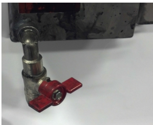
Waste Tank Valve in closed position
