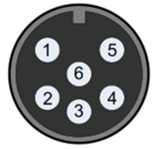
6-Way, Female, Lumberg View from Solder Side
