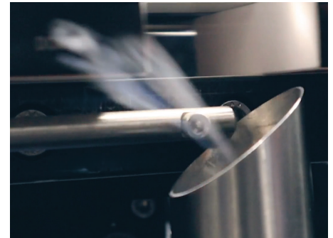
Domino's DPX fume extraction systems effectively filter fume and particulate debris from the coding process.
