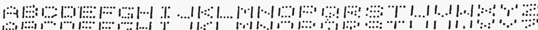
Printing drops clipping edge of gutter – jet incorrectly aligned to gutter, or print height too low
