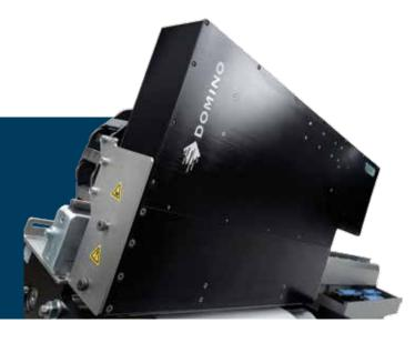
The **K6**00i is a world leader based on the Generation 6 technology with more than 600 global installations. Available with high impact UV-curable inks as well as cost effective aqueous pigmented inks, this inkjet press can operate at speeds of up to 200/min. Offering your customers added-value and increasing their sales and profitability.
